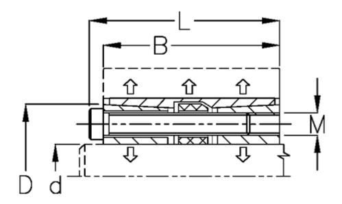
$\begin{array}{lll} \text{B mm} & = 122 \\ \text{d H8 mm} & = 100 \\ \text{D mm} & = 145 \\ \text{Fit tolerance} & = \text{Aksel h8, Nav H8} \\ \text{F kN torque} & = 570 \\ \text{L mm} & = 134 \\ \text{M mm} & = \text{M12} \\ \text{P N/mm2 surface pressure on shaft/hub} = 80 \end{array}$
